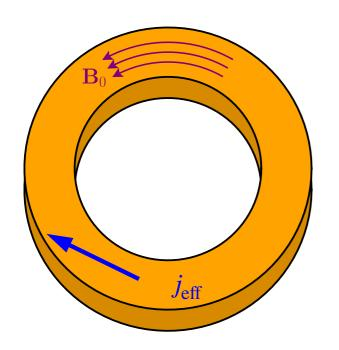
At the interface of two bodies with different values of the magnetisation vector M, Maxwell's equations predict a surface current proportional to  $n \times \Delta M$
