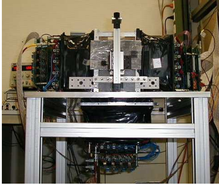
Figure 6.23: Prototype employed in the second run. Two scintillators are placed on both sides and below the scatter detector, that is inside the metal box.
