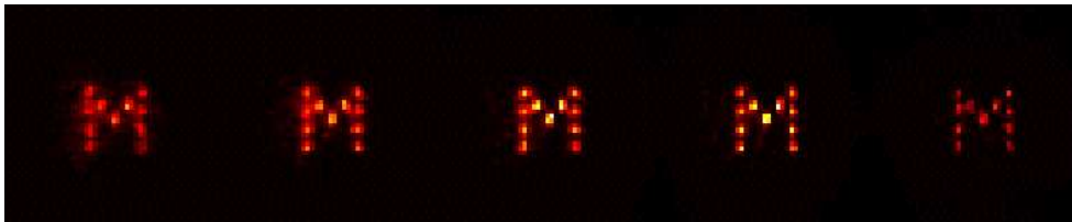
Figure 4.3: Reconstruction of a M-shaped array of point sources with the endorectal probe configuration at different energies. From left to right, 140.5 keV ( ^{99m}\text{Tc} ), 171 keV and 245 keV ( ^{111}\text{In} ), 364.4 keV ( ^{131}\text{I} ), and 511 keV ( ^{11}\text{C} )
