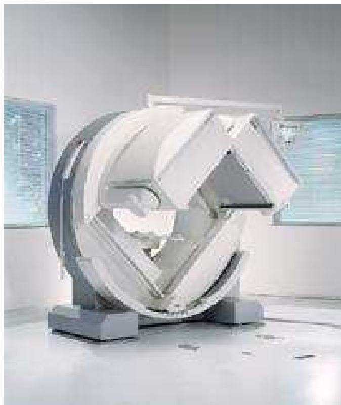
Figure 1.1: SPECT system with two imaging heads at 90 degrees to each other.
