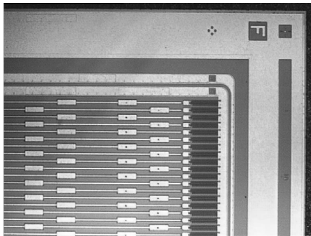
Fig. 3: Photograph of a corner of an SCT barrel silicon microstrip sensor, showing the guard structure, a selection of fiducial alignment marks, the bias ring, polysilicon resistors, and the metallization above implant strips, including wire-bonding pads.
