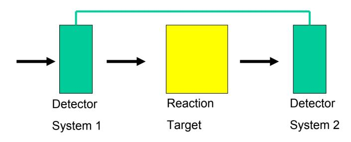
2. Special ion optical systems (Energy-loss spectrometer)
