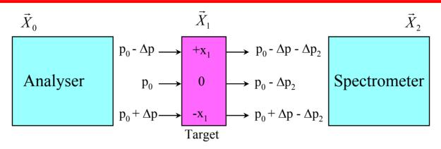
Point - to - point image condition: ( $R_{12} = (x, x') = 0$ )
