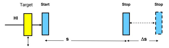
1. Time of flight measurement in a free drift space
