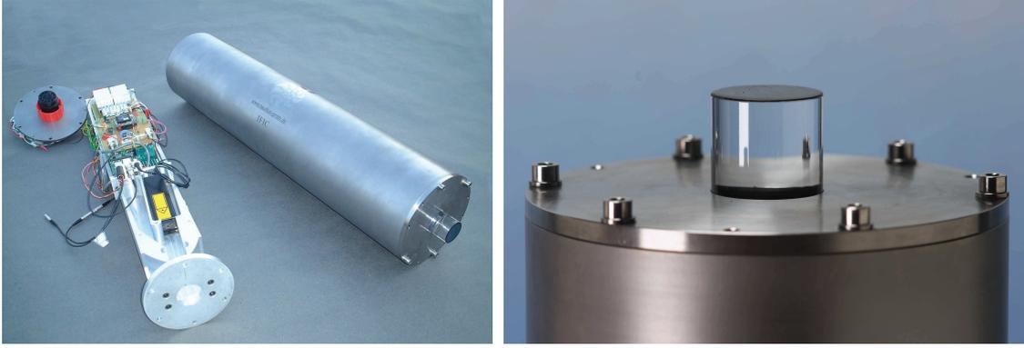
Figure 3.2: *left*, the Laser OB and its titanium container; *right*, detail of the upper end-cap of the Laser OB with its antibiofouling quartz rod system.
