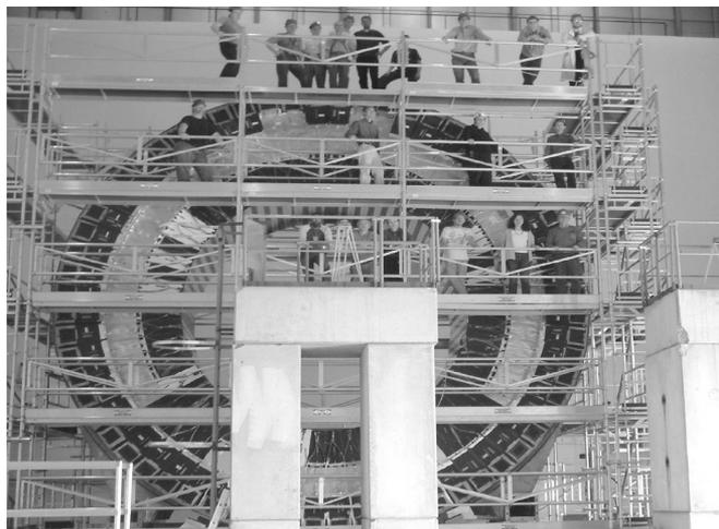
Fig. 3. The first completely pre-assembled extended barrel of the Tile Calorimeter placed behind the scaffolding.
