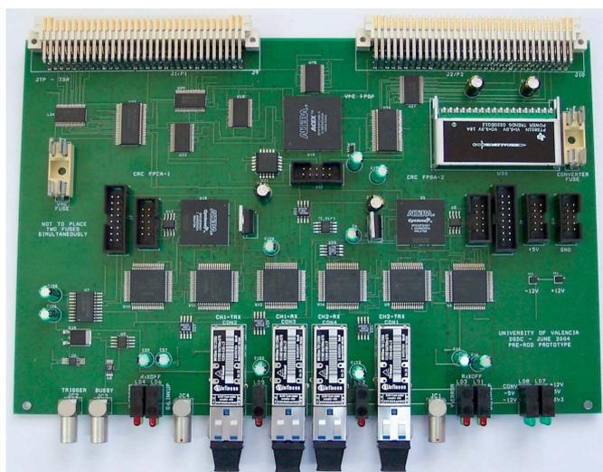
**Figure 6.** The optical multiplexer board prototype.
