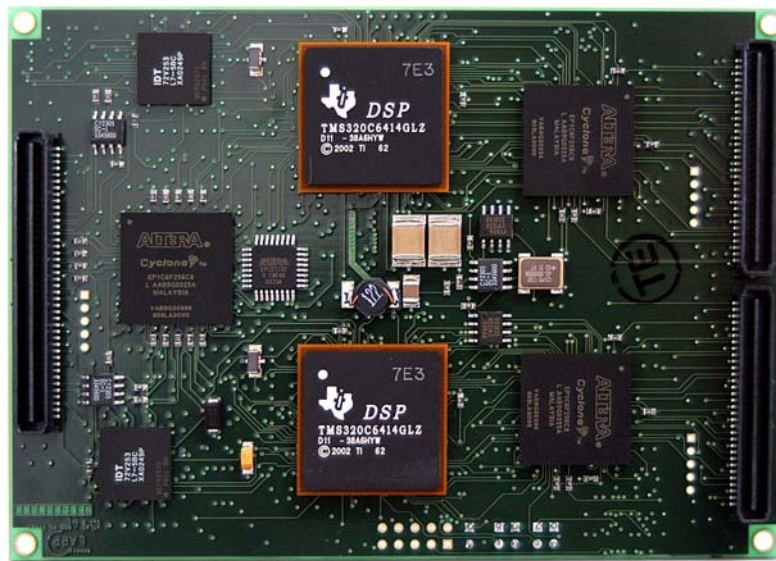
Figure 5: Picture of the DSP PU.
