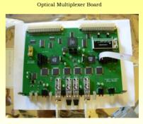
TileCal is a redundant data acquisition system. Two optical fibers carry the same data from the front-end electronics to the ROD. This is necessary because of radiation phenomena which could cause malfunctions inside the front-end electronics, and bit and burst errors over data ready to be transmitted to the ROD card.
