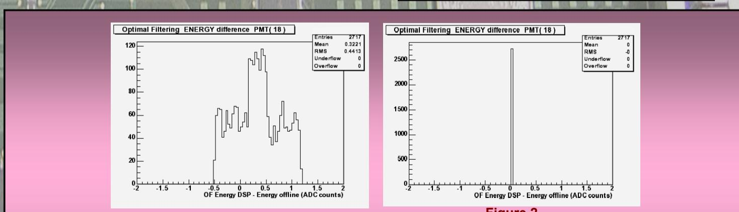
Figure 1 shows the difference between the Amplitude calculated online in the DSP and the Amplitude calculated offline, working in floating point and with 32 bits words.
