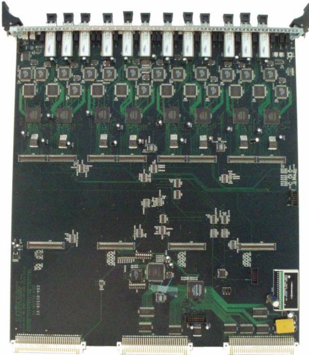
Fig. 5. Picture of the OMB 9U prototype board.
