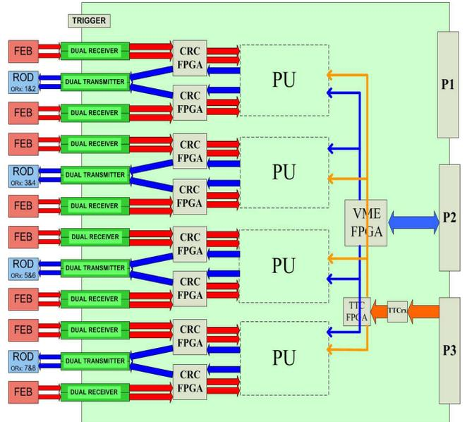
Fig. 11. Dataflow of the OMB 9U prototype. PU processing mode.
