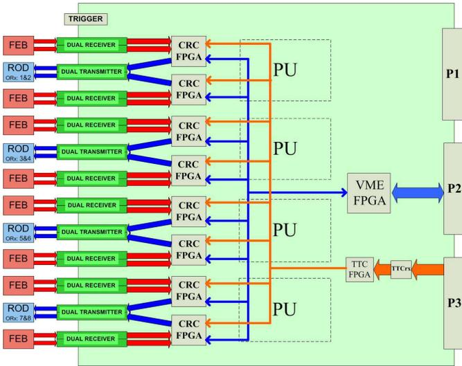
Fig. 9. Dataflow of the OMB 9U prototype. CRC checking operation mode.
