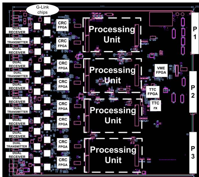
Fig. 8. OMB 9U prototype main components.
