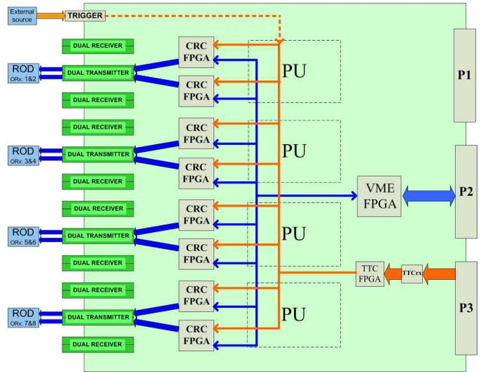
Fig. 10. Dataflow of the OMB 9U prototype. Injection mode.
