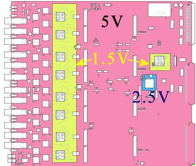
Fig. 7. Power distribution in the internal layer number 9.
