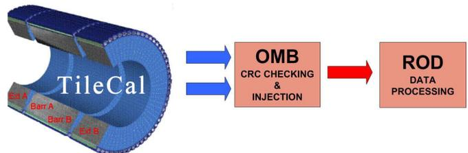
Fig. 2. The OMB in the TileCal data acquisition chain.
