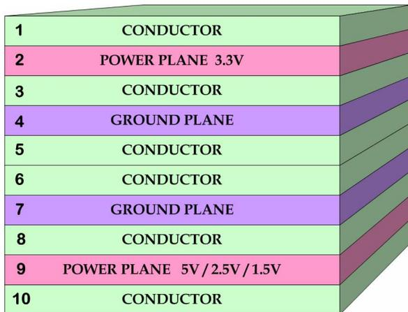
Fig. 6. OMB 9U prototype layer stackup.
