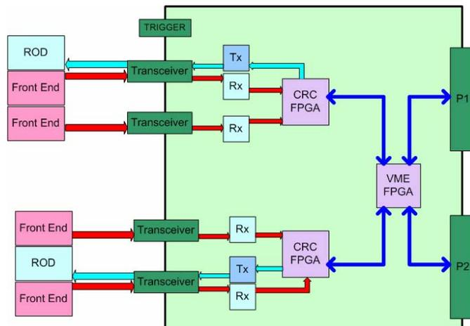
Fig. 4. Diagram of the OMB 6U dataflow.
