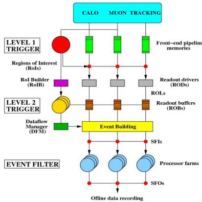
Fig. 1. The ATLAS three levels trigger system.
