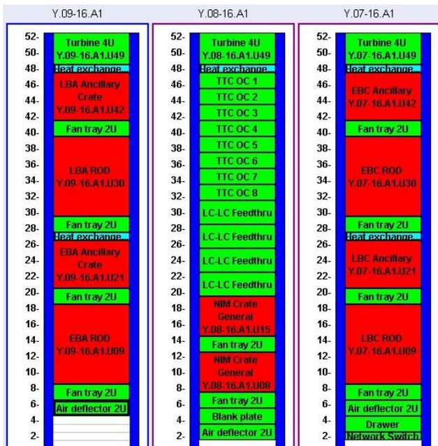
Fig. 3. TileCal back-end electronics racks distribution.
