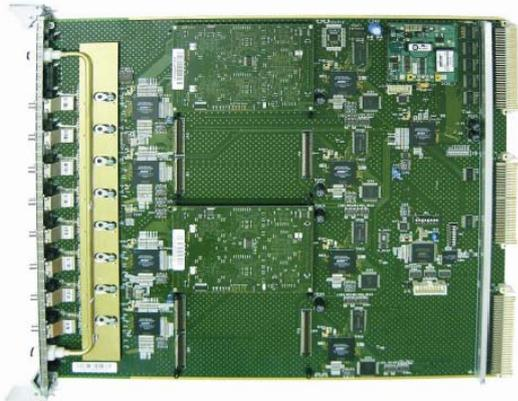
Figure 1: ROD motherboard with 2 Processing Units.
