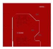
Figure 6: PWR2 split power layer detail.
