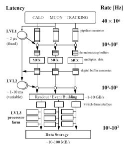
Figure 1: The ATLAS three levels trigger system.
