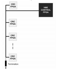
Figure 7: First routing scheme from VME to CRC FPGAs.
