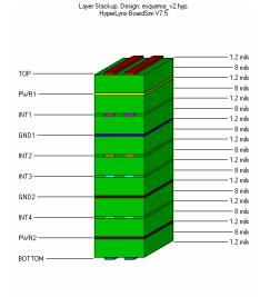
Total thickness = 84 mils Figure 5: OMB 9U Prototype layer stackup.
