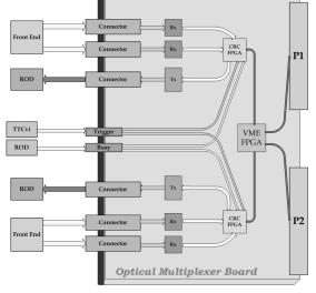
Figure 2: Optical Multiplexer Board Block Diagram.
