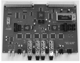
Figure 3: The Optical Multiplexer Board prototype.
