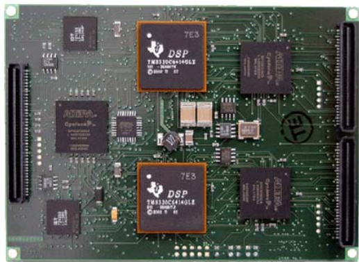
Fig. 9. Picture of the back side of the Processing Unit used in the ROD with two Digital Signal Processors.
