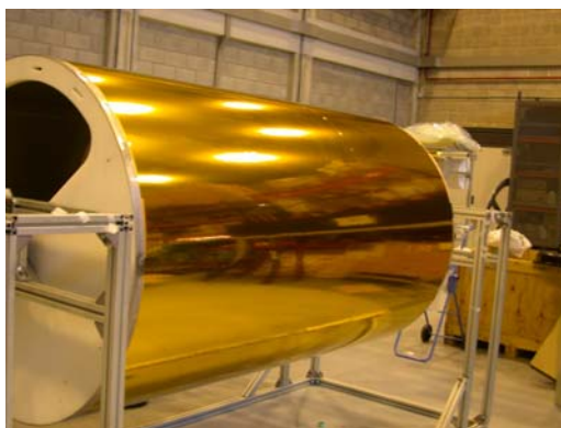
Fig 15. Al-k inner layer placed on the mandrel. Two sheets used to cover the length.
