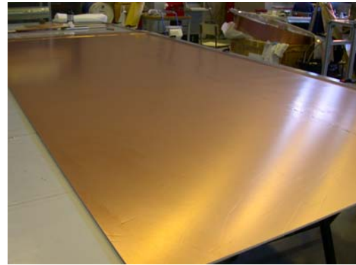
Fig 12. Cu-k layer already glued to Airex substrate.
