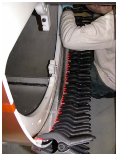
Fig 19. Tweezers used for gluing one CF sector of the Front Flange.
