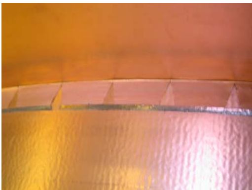
Fig 21. Soldering of the Cu-k tabs to the Cu-k layer of the cylinder.
