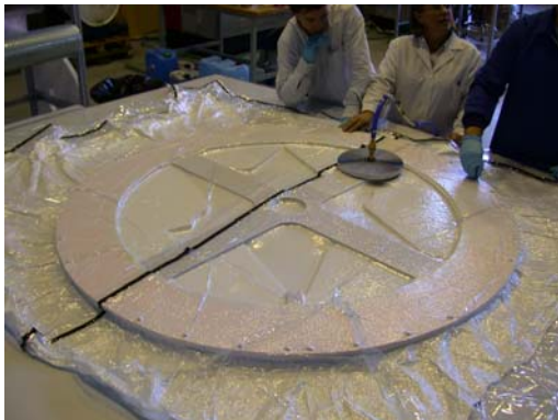
Fig 8. Placing the Cu-k layer onto the Airex sheet covered with glue.
