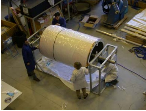
Fig 14. Main cylinder assembly. Vacuum used on the mandrel
