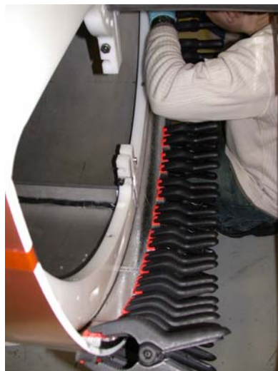
Fig 16. Tweezers used for gluing one CF sector of the Front Flange.
