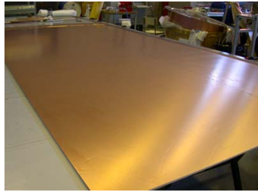
Fig 9. Cu-k layer already glued to Airex substrate.
