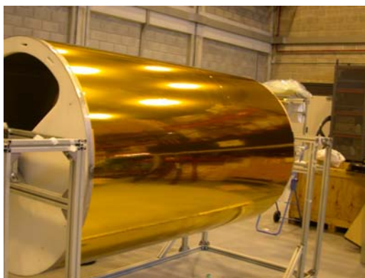
Fig 12. Al-k inner layer placed on the mandrel. Two sheets used to cover the length.
