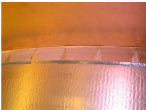
Fig 18. Soldering of the Cu-k tabs to the Cu-k layer of the cylinder.
