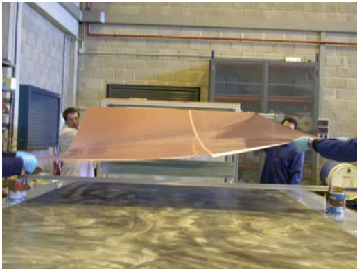
Fig 8. Placing the Cu-k layer onto the Airex sheet covered with glue.
