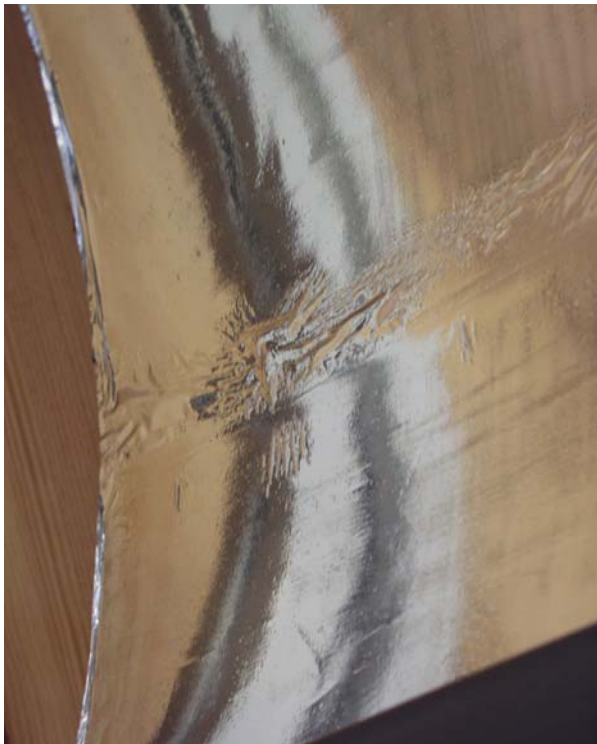
FIG 6 Imperfections on inner surface.
