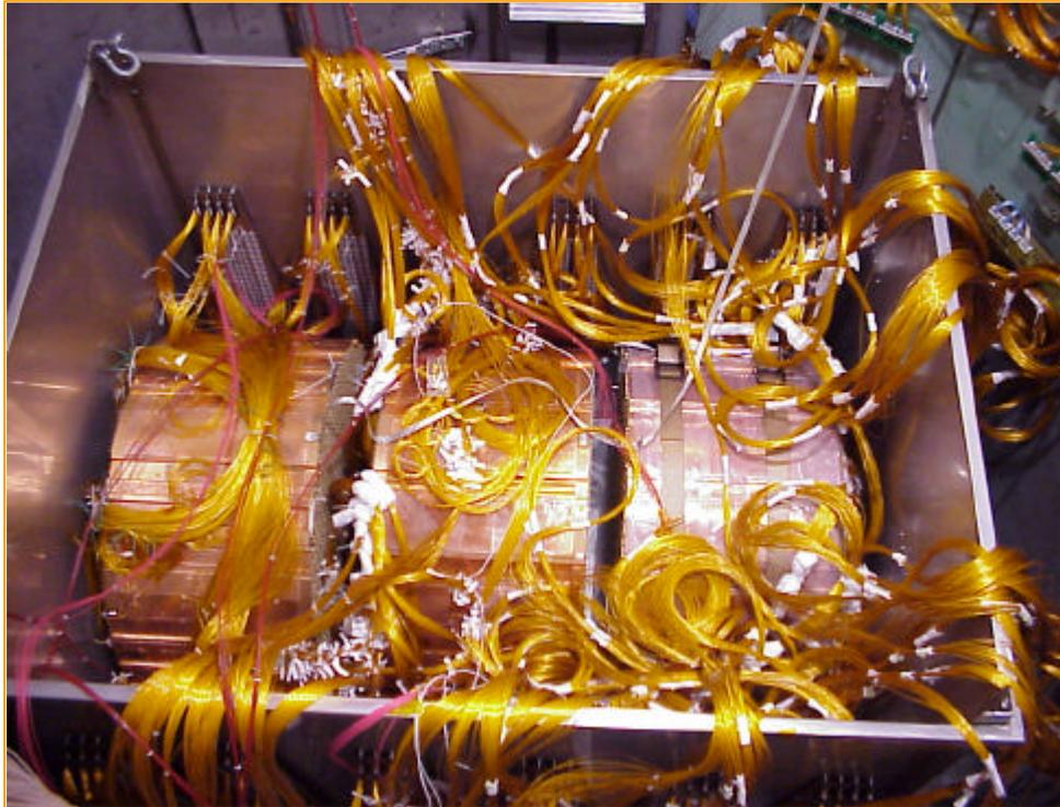
Cold test of the three FCAL modules for the first side
