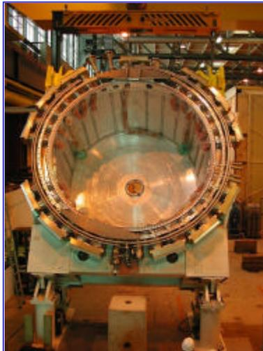
Cryostat ready for detector installation
