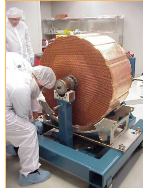
FCAL module during insertion of W rods
