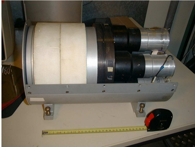
Figure 2.11: Photo of the larger NaI(Tl) crystal of the TAGS detector. This part of the detector has a longitudinal hole of \varnothing = 43 mm.
