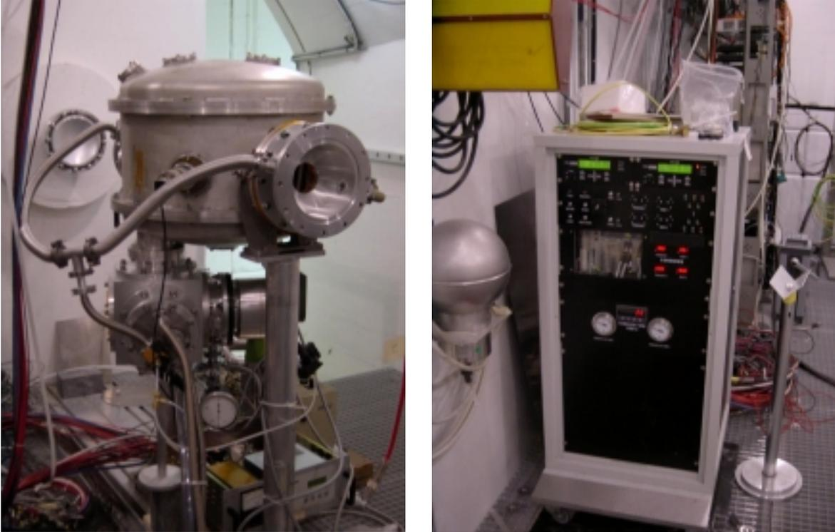
**Figure 3-4:** The vacuum chamber of the PPAC detectors (*left*) and the associated gas and safety control unit (*right*).
