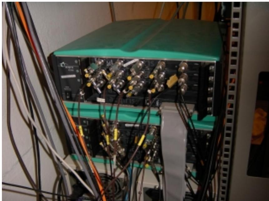
**Figure 2-3:** The ACQIRIS digitiser modules and the chassis.
