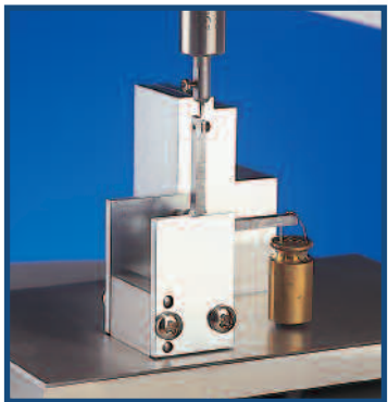
Automatic load cartridge calibration using traceable weights.
